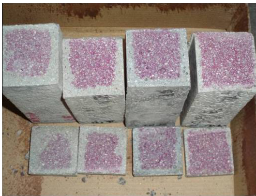
Fig. 4. Carbonation depth measurement by spraying with phenolphthalein indicator.
