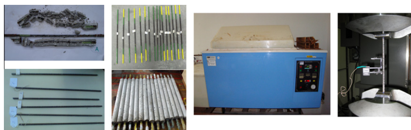
Fig. 2. Salt spray exposure chamber, preparation and testing of steel samples.
