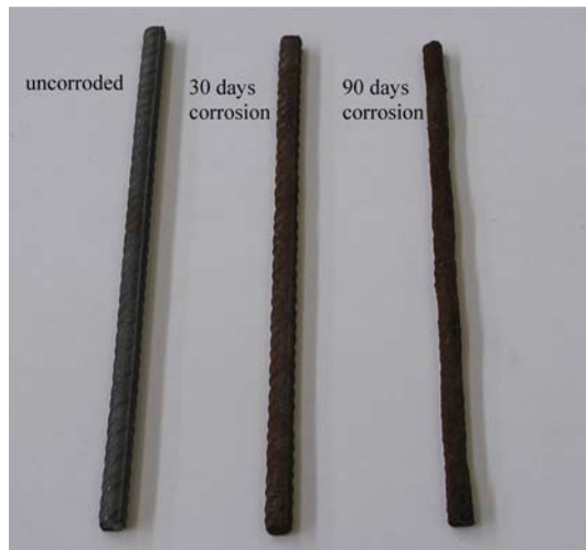
Fig. 4 Uncorroded steel bar (left) and steel bars after 30 days (middle) and after 90 days (right) exposure at a chloride-rich environment
