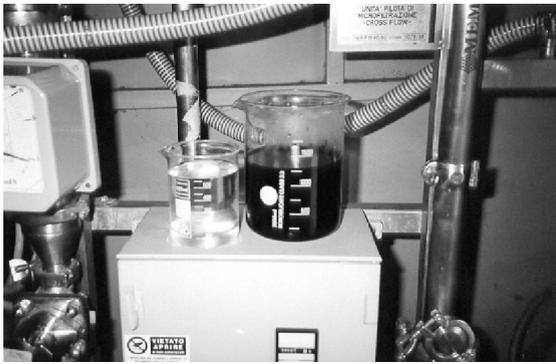
Fig. 3. Photograph of samples before (right cylinder-feed) and after nanofiltration process (left cylinder-permeate).
