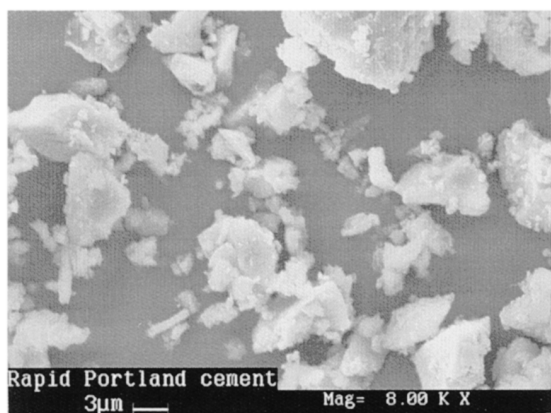
Fig. 1. SEM micrographs (8000×) of Portland cement (left) and silica fume (right).
